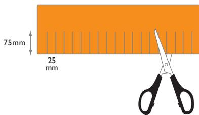
**5** Cut another piece of matting with a rough semi-circle slightly smaller than the pipe circumference cut out. Repeat this for the other side.
