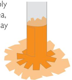
**9** Now place one of the pieces of matting over the fanned out matting on the roof deck and paint over with resin. Repeat for other side.
