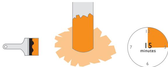
**8** Whilst resin is still wet apply matting over wetted in area, leaving the 25mm cuts to lay on the roof surface and then brush more resin over matting, ensuring you cover all the matting.
