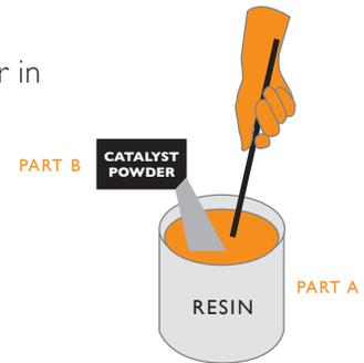
**7** Time to work quickly - first liberally apply pre-mixed resin around pipe and to repair area making ready to receive matting. You have approximately 15 minutes total working time.
